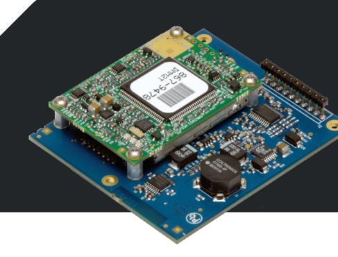
The FreeWave MM2-MR radio has been designed to provide the performance, reliability, and quality that our customers have come to know and expect in our products in a MM2 "Mega Mini" form factor for applications where space is at a premium. The MM2-MR has all of the functionality of the larger footprint FGR2 Series of radios.
