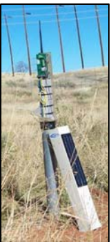
FGRCP LineMarker Test Station Available with one or two solar panels.
